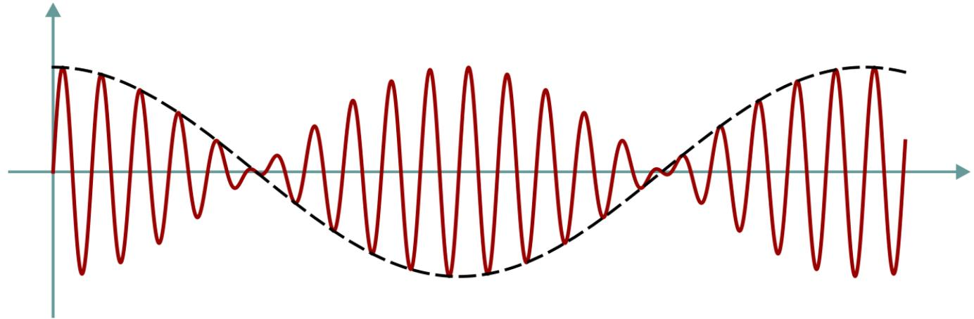
$$S = 2A \cos\left(\frac{\omega_2 - \omega_1}{2} t\right) \cdot \cos\left(\frac{\omega_2 + \omega_1}{2} t\right) = 2A \cos\left(\frac{\Delta\omega}{2} t\right) \cdot \cos \omega t$$
